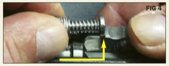
Push simultaneously back and forth to compress the Recoil Rod and pull it up to release it from the barrel link (Fig. 5).
