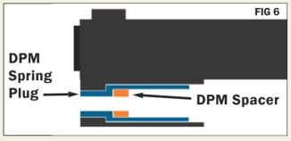
The DPM Recoil System includes 4 different powered springs and 3 different sized spacers so the user can fine tune the opening and locking position forces on the pistol's slide. (Fig.7)
