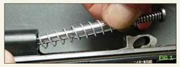
2. Continue pushing the Recoil Rod from the back side. FIG 2
