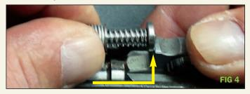
Push simultaneously back and front to compress the recoil rod and pull it up to be released from the barrel link. FIG 5
