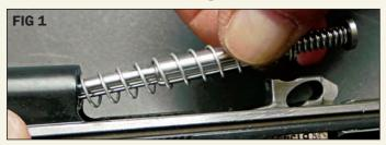
2. Continue pushing the Recoil Rod from the back side (Fig. 2).
