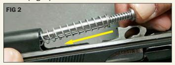
Finally push the Recoil Rod, until the front side passes through the slide hole and press down to lock the back side of the rod on the barrel link (Fig. 3).
