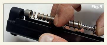
**3.** Insert the DPM Washer in the slide pistol and then insert the DPM Recoil System with an External Spring of your choice. (**Fig. 6 & 7**)
