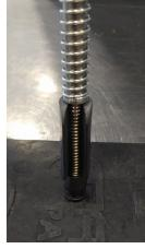
Step 1: Adjust the Distance Tool on the Recoil Rod and set the base of the Rod on a non-slippery surface. Fig. 1
