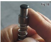
Make sure that the Safety Pin's edges after the installation are within the Recoil Rod and not outside of it.
