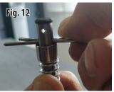
**Step 4:** Insert the Locking Pin to the Assembling/ Disassembling Tool in Option 2, set on a table the Recoil Rod and push to insert complete in to the hole. **Fig 13, 14 & 15 Step 5:** Remove the Safety Pin, and push down the Ex-
