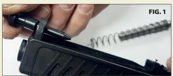
1. Choose one of the DPM external springs and install it on the recoil rod. Insert the assembling tool from the front side of the slide hole. (FIG. 1)
