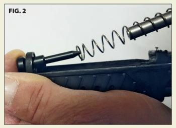
Insert the edge of the spring in the tip of the assembling tool. (FIG. 2)
