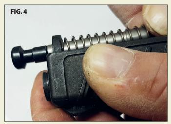
Release the assembling tool and push until the recoil rod passes a little from the slide hole. (FIG. 4)
