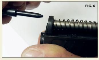
Remove the Assembling Tool. (FIG. 6)
