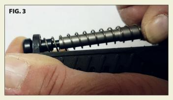
Hold the assembling tool firmly with your index finger on the slide hole. Then push the recoil rod so the tip of the assembling tool to be fully inserted in the rod. (FIG. 3)
