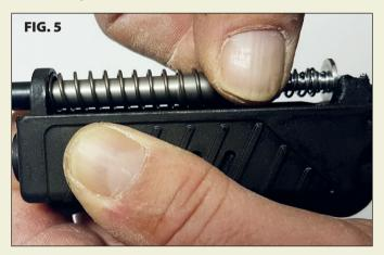
Align the recoil rod and let it sit on the barrel rod position. (FIG. 5)
