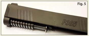
4. Ensure that the DPM system is placed in the correct way, reassemble the slide on the frame and rack the slide several times to ensure that the DPM Recoil system functions unrestricted.
