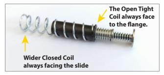
With the Wider Coil facing the Slide, Push from the middle section, until the rod will pass through the Slide hole a few milimeters. (Fig. 1 & Fig. 2)
