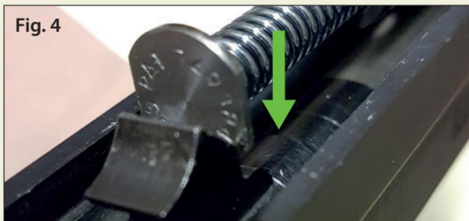
3. Ensure that the DPM system is placed in the correct way, reassemble the slide on the frame and rack the slide several times to ensure that the DPM Recoil system functions unrestricted.
