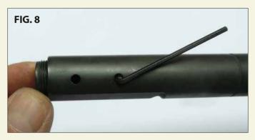
**6.** Attention! Remove the allen tool to release the DPM buffer and the main spring. **FIG 9**Now you are ready to add the stock on your shotgun.
