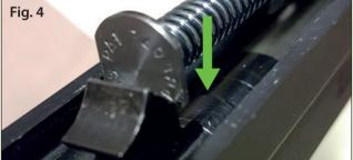
3. Ensure that the DPM system is placed in the correct way, reassemble the slide on the frame and rack the slide several times to ensure that the DPM Recoil system functions unrestricted.
