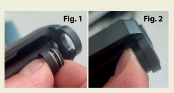
2. Insure that the plug is placed correctly. Fig. 2
