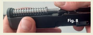
**6.** Assemble the pistol and rack the slide a few times to check fon any unseen interferences and to ensure that the DPM Recoil System operates unrestricted.
