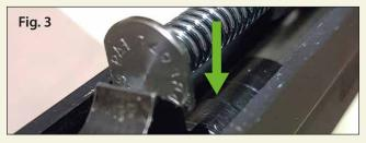
3. Ensure that the DPM system is placed in the correct way, reassemble the slide on the frame and rack the slide several times to confirm that the DPM Recoil system functions unrestricted.
