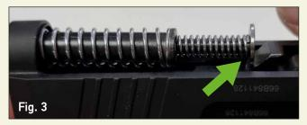
POWER RATES Slide in battery (idle position): 9 lbs Slide at full open position: 12 lbs
