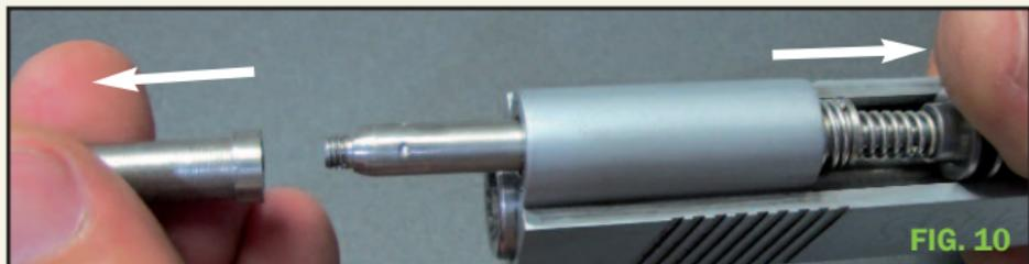
**Assemble the Slide on the Frame and function (open and close) the slide several times by hand to Ensure that the DPM Recoil Reduction System operates unrestricted.**
