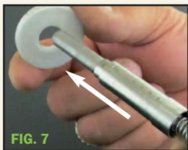
**7. Remove the Compressive Disc and the Recoil Rod is now ready for installation. FIG. 7**
