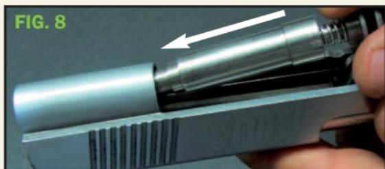
**8. Insert the Recoil Rod in the Pistol Slide. FIG. 8**
